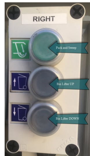
Figure 3 Bin Lifter Controls
