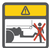
Danger of crushing due to underride protection / Don't step here
