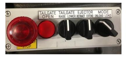
Mode In the Load position enables the Compactor and Bin Lifter functions only to
