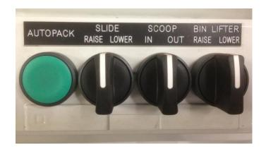
Auto pack Starts compaction cycle. Compaction cycle will stop when slide blade has
