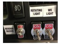
Work Light Toggle switch for turning on the work light to illuminate the Hopper and Bin
