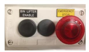
Bin Lifter Enable Button must be depressed simultaneously with Bin Lifter - Lower / Raise
