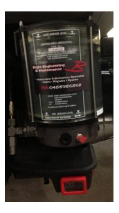
The grease to be used MUST be an EP2 NLGI2 grade grease with no more that 2.5% Moly content A recommended brand is IMXO2 grease
